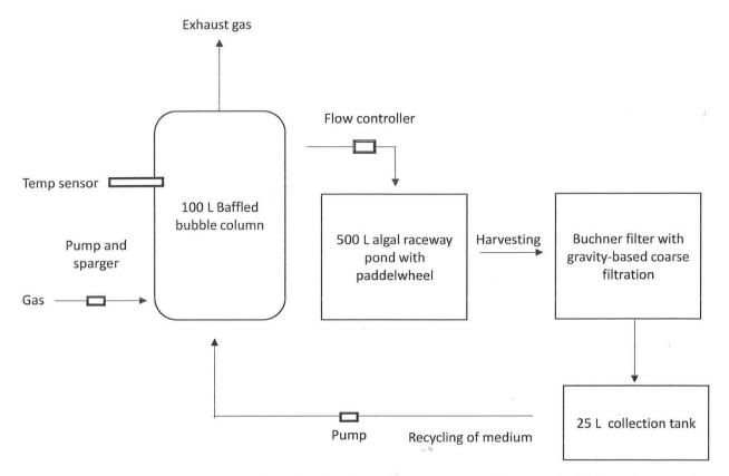
**Schematic:** CO2-enriched gas will be absorbed in the culture medium in bubble column. The medium will then be supplied to raceway pond for algal growth.
